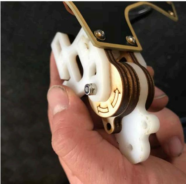
The bolts should easily fall into place if the nut holder is correctly aligned.
